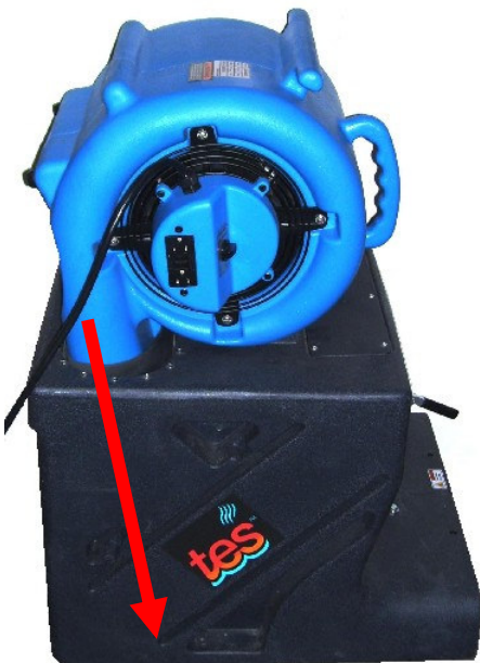
Snout Not Angled Properly
